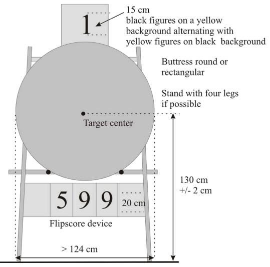
Image 4: Indoor target butt set-up.
