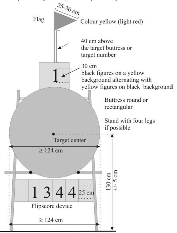
Image 3: Outdoor target butt set-up.
