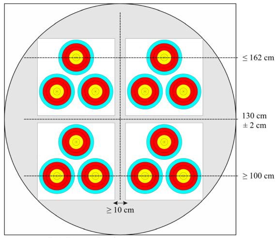
Image 8: 4 x 4 Triple Triangular Face for Indoor.
